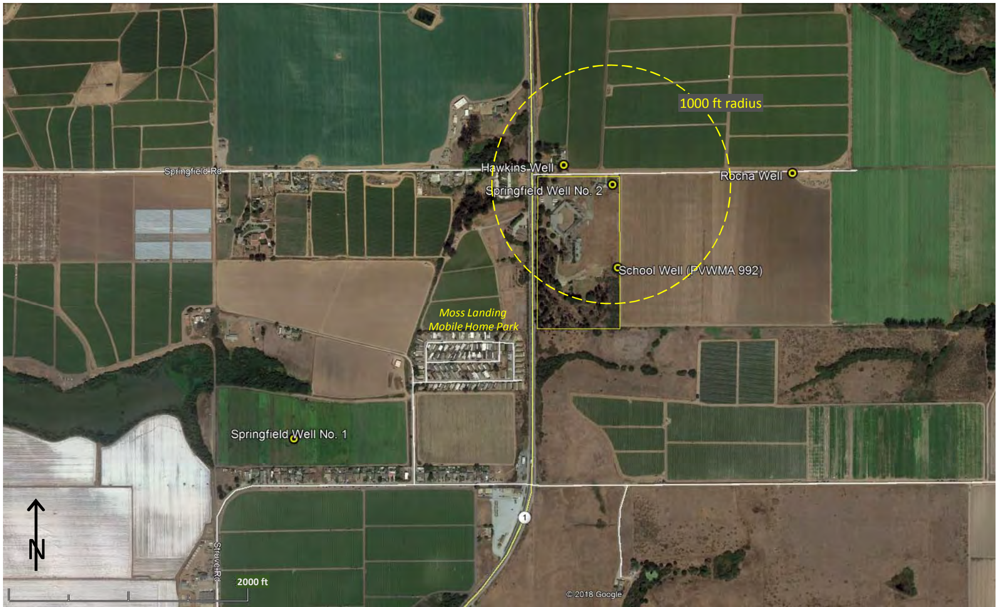
Figure 14. Test well no. 2 relative to neighboring wells, Springfield water system, Pajaro / Sunny Mesa Community Services District, Monterey County, California.
